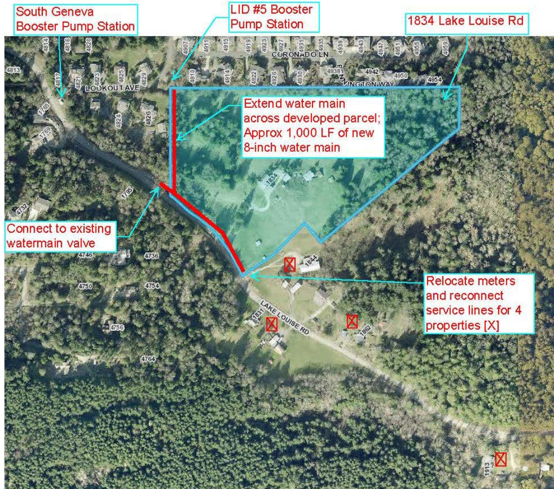
Figure 1. Lake Louise Road Short Plat Water Supply Schematic
