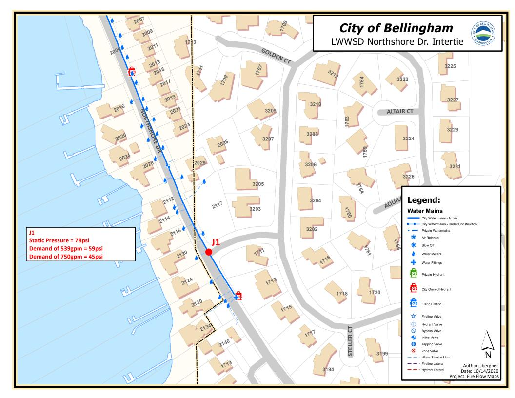
One thing we discovered as we were digging in is that the Eagleride fire flow standard is actually 500 gpm, not the 750 gpm we previously discussed. Could you re-check your scenario (where you got 45 psi at 750 gpm), and tell us pressure at J1 under 539 gpm (500 gpm fire flow plus 39 gpm MDD)?
