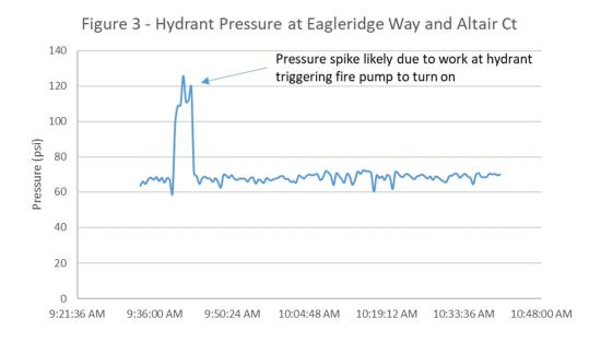
Since it appears that the fire pumps will remain necessary, we recommend replacing them with appropriately sized pumps (based on current suction-side pressures and fire flow needs) with VFD controls.
